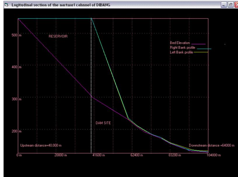
Fig. 15.3: Channel bed and computed flow profiles
