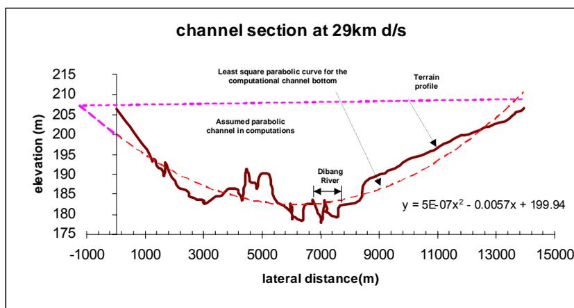
Fig. 15.6: Approximated channel section
