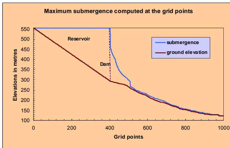
Fig. 15.11a: Sectional view of maximum Submergence
