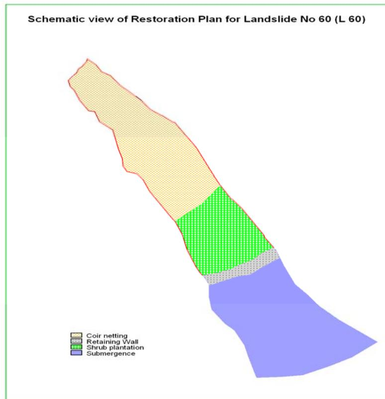
Fig. 7.3: Schematic view of restoration plan for landslide L 60
