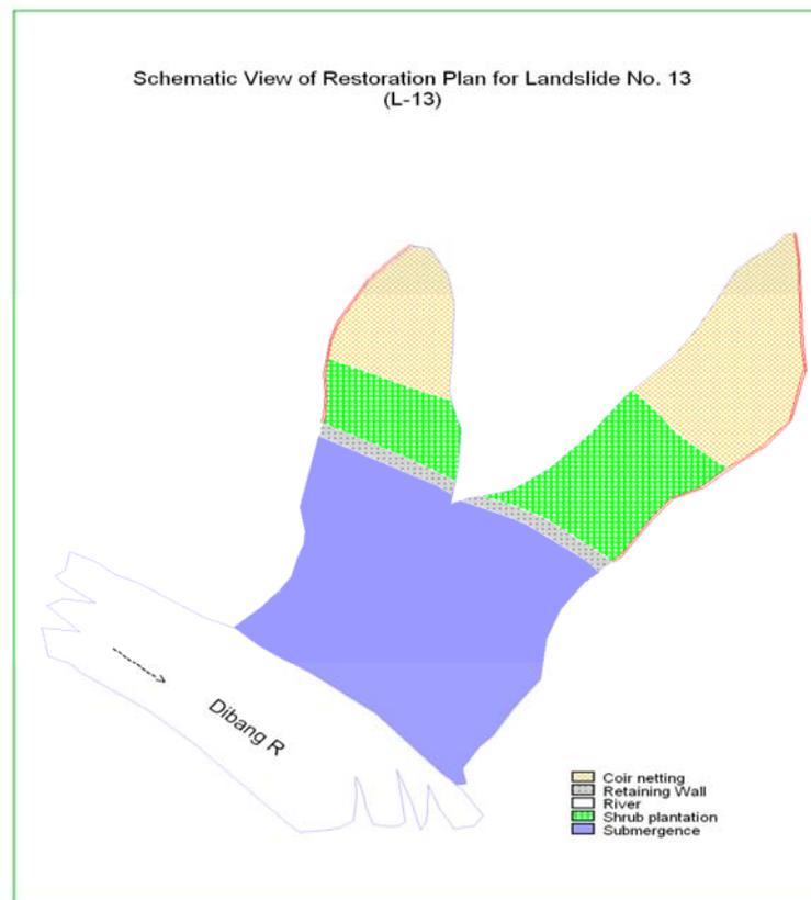
Fig. 7.5: Schematic view of restoration plan for landslide L 13
