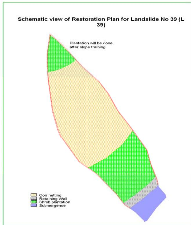
Fig. 7.4: Schematic view of restoration plan for landslide L 39
